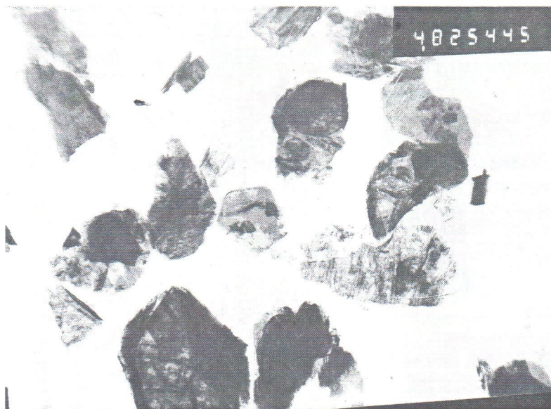
Figure 6.5. TEM micrograph of shock synthesized w-BN (4000 \times )
