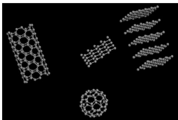
Solid Lubricants, Graphene, Fig. 1 The schematics of graphene ( middle, upper ), fullerene ( middle, lower ), carbon nanotubes ( left ), and graphite ( right )
